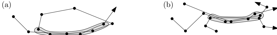
Figure 1: (a) The two subtrajectories within the shaded region form a subtrajectory cluster for m = 2 if the length of the longest subtrajectory is longer than \ell and the Fréchet distance between the two subtrajectories is at most d . (b) Illustrating a subtrajectory cluster for m = 3 in the case when a set of trajectories is given as input.
